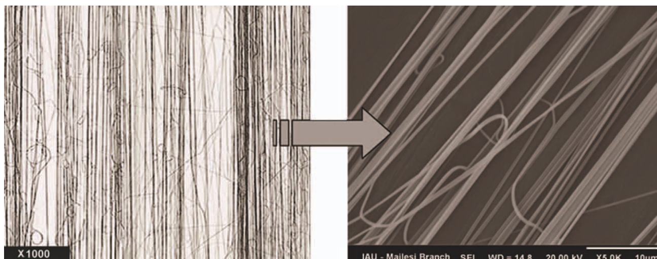
Figure 2 Unidirectional bundles of aligned PAN nanofibers collected on rotating drum. [Color figure can be viewed in the online issue, which is available at wileyonlinelibrary.com .]
